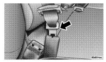
**Inserting Latch Plate**
